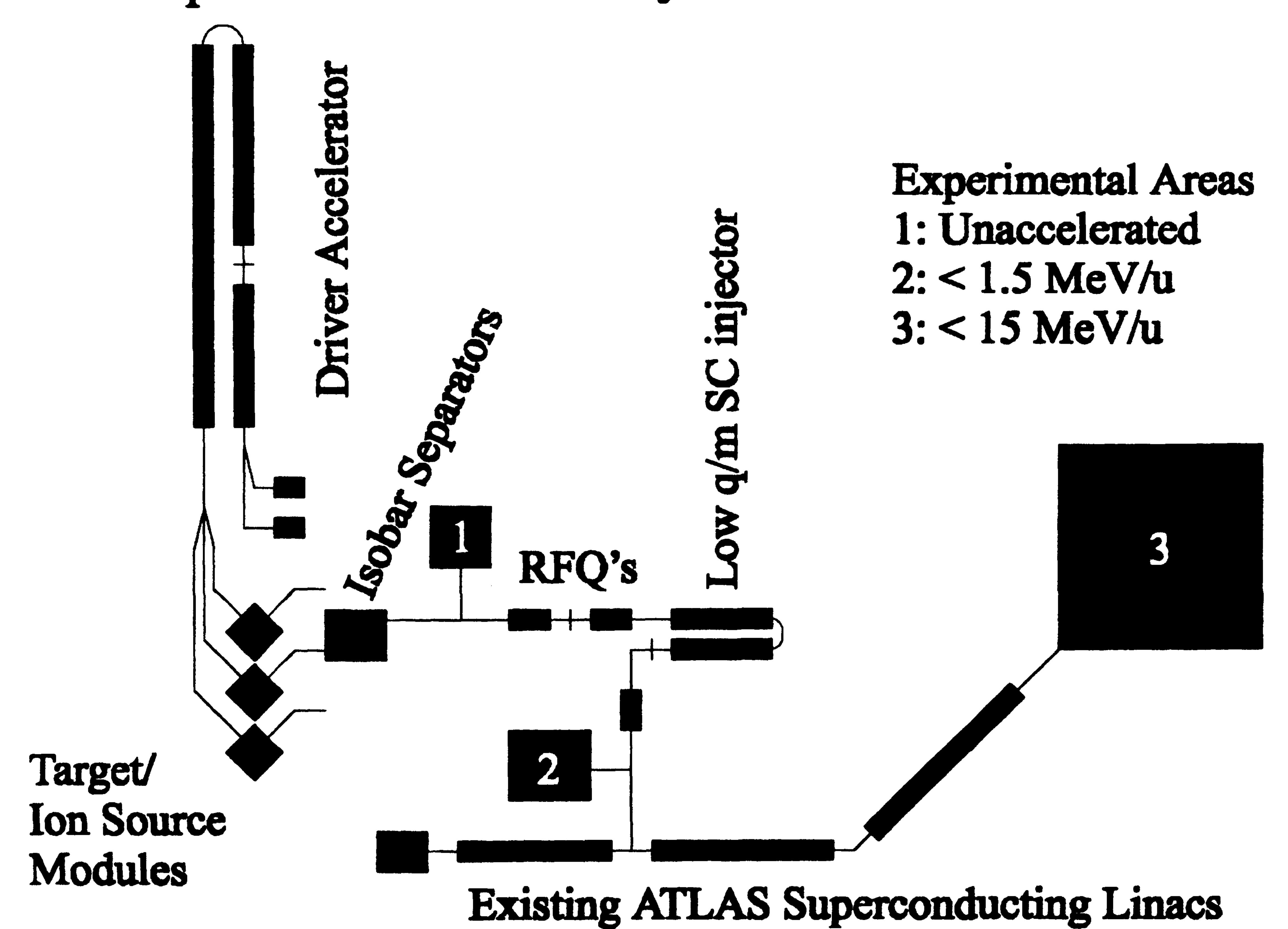
FIGURE 1. A block diagram of the proposed Advanced ISOL Facility based on ATLAS at Argonne. The major components of the complex, including the three different experimental areas, are indicated. The details of the low energy beam switchyard that connects the three target modules to the various experimental areas and/or post accelerators are not shown.
