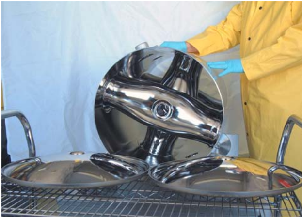
Figure 2: Major niobium subassemblies of the \beta=0.62 triple-spoke resonator after final electropolishing
