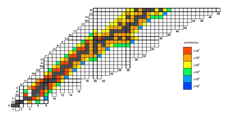
Estimated rates for rare-isotope beams at the exit of AIRIS (rates are uncertain by as much as one order of magnitude). They assume primary beam parameters of 10 MeV/u and 1 particle- $\mu$ A, a ~1 mg/cm² production target, estimated reaction cross sections, the dominant charge state fraction, and transmission through AIRIS.
