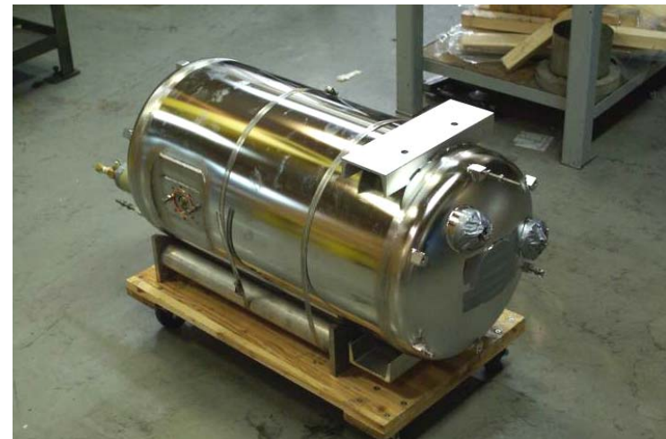
Cavity housing/Cryogenic vessels
