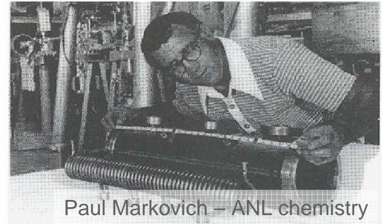
Helical Nb resonator developed at ANL for a heavy-ion linac.
