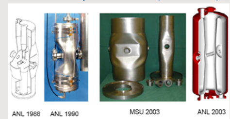
TEM \lambda/2 - \beta \sim 0.12-0.2 (\sim 200\text{MHz})
