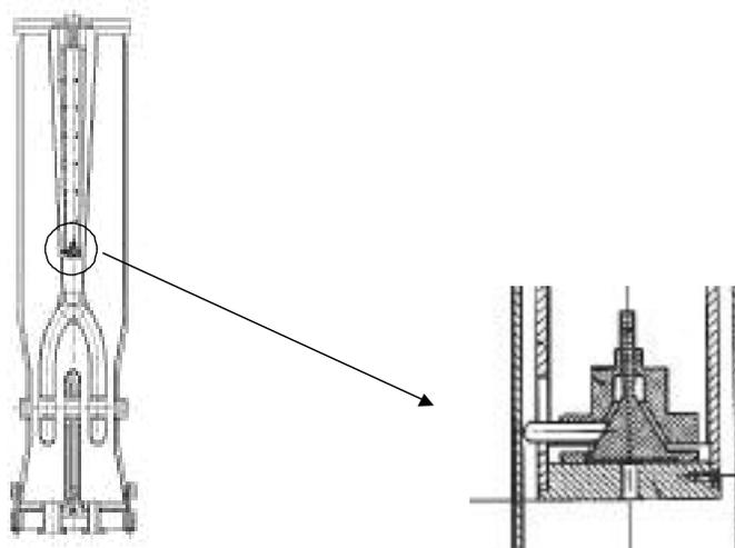
Figure II-3. Components of the Vibration Damper
