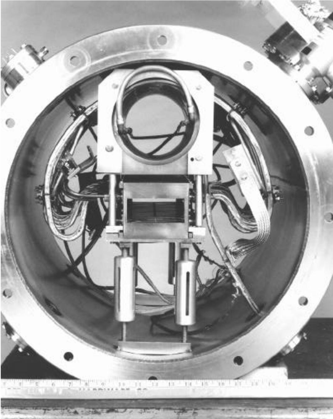
*Figure II- 4. Photograph of the assembled transmission-line chopper in its vacuum housing. Shown is a portion of the semi-rigid delay-lines connecting the sequential electrodes visible in the rectangular beam aperture.*
