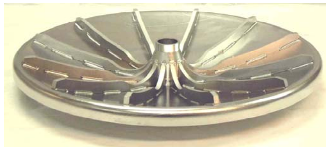
Fig. III-2. Niobium end-cap assembly for the prototype two-cell cavity after welding.
