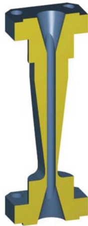
Fig. III-33. A cutaway view of the beryllium target spool piece for the hybrid target. The beryllium entrance and exit windows vary from 1-mm thick at one end to 7-mm thick at the other. Lithium flows between the windows and is 5 mm thick. The overall target varies from 0.7 \text{ g/cm}^2 to 3 \text{ g/cm}^2 .
