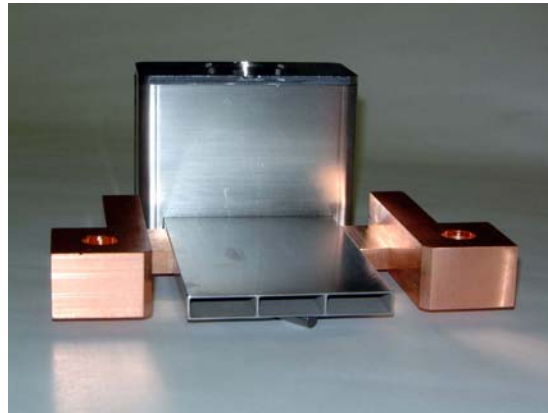
Figure III-20. Photograph of the pump duct and current electrodes for the prototype target.
