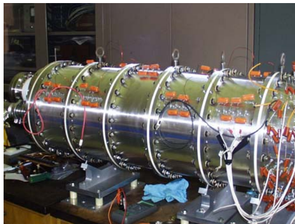
Figure III-32. View of the capacitors and resistors connected to the internal electrodes to feed the DC and RF fields and that form part of the tank tuned circuits.
