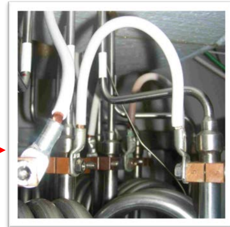
Direct heating of GC columns (60 A)
