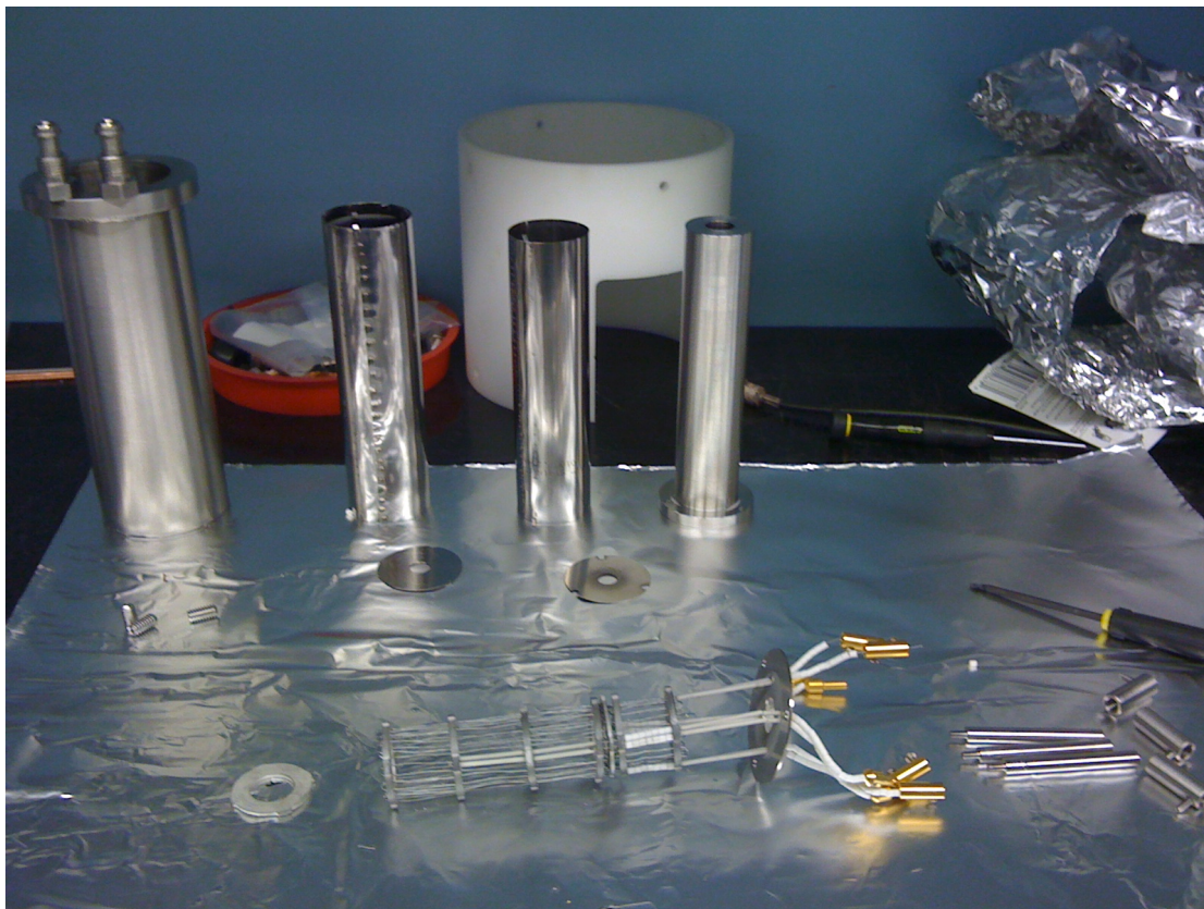
FIGURE 4.6: Disassembled oven, showing the component parts. The upper part of the image shows the stainless steel heat shields; the leftmost shield has feedthroughs for water cooling. The bottom shows the two oven filaments, a long one in front and a short one in the back, which (when assembled) surround the oven nozzle and heat it radiatively (the filaments are supported on ceramic spacers to avoid direct contact with the oven nozzle and crucible).
